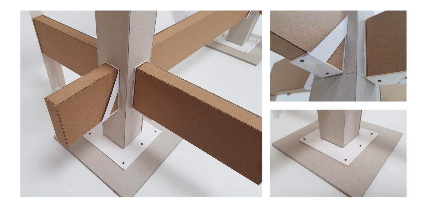
The Model: This physical handmade 1:20 Detail Model is of a timbre beam and concrete wall connection. It was made using a range of materials such as Grey board (Concrete), White Mount board (Steel), Cardboard (Timbre) and Nails (Screws) to signify the concrete foundation and column held together with a steel plate, and timber beams being supported onto the column with a metal beam hanger.
